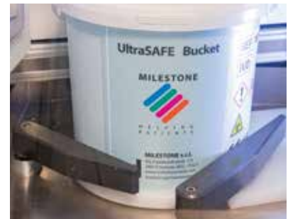
The bucket is automatically centered and the weight of the biospecimen is detected
