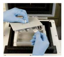
7 Slide the cryomolds from the holder.
