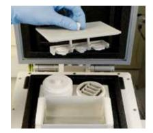
6 After the freezing time has expired, take out the slide-in holder.
