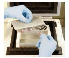
4 Position each cryomold in the slide-in holder.
