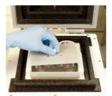
5 Place the slide-in holder on top of the tank. The fluid inside the set level tank freezes only the mold without contaminating the specimen.
