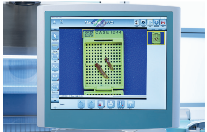
C-Scan reads the cassette's code, creates the respective case ID folder and takes a picture at a preset zoom.
