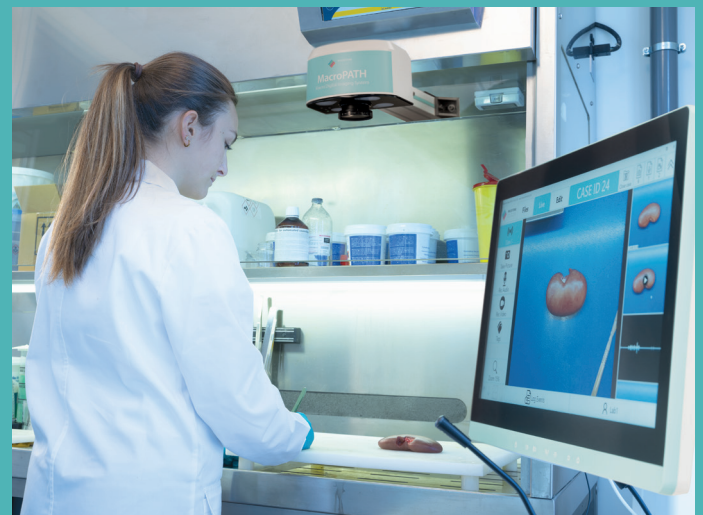
MacroPATH installed on an existing grossing station
