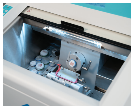
White LED confirms normal operation
