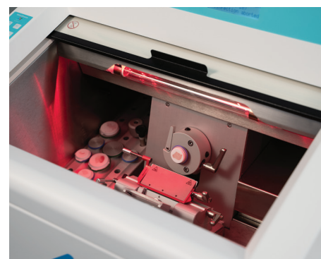
Red LED indicates an error
